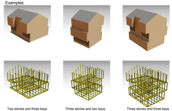
Fig. 4 Smart BIM test with different surface model input.
